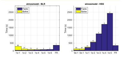
Comparatively with BLR, HSS favors low-accuracy preconditioning Applying improved preconditioner to HSS (or fully-structured BLR) should have an even greater impact! Accuracy and Stability of Low-rank Solvers Theo Mary
