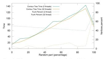
Figure 9: FTC contour tree computation time for 2 and 32 threads on our worst case data set as the random part progresses form 0 to 100% (plain lines, left axis) and percentage of vertices processed by the trunk procedure (dashed lines, right axis).
