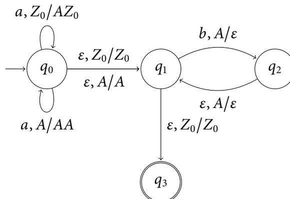
Exécution de l'automate :  $(q_0, aaaabb, Z_0) \vdash (q_0, aaabb, AZ_0) \vdash (q_0, aabb, AAZ_0) \vdash (q_0, abb, AAAZ_0) \vdash (q_0, bb, AAAAZ_0) \vdash (q_1, bb, AAAAZ_0) \vdash (q_2, b, AAAZ_0) \vdash (q_1, b, AAZ_0) \vdash (q_2, \varepsilon, AZ_0) \vdash (q_1, \varepsilon, Z_0) \vdash (q_3, \varepsilon, Z_0)$ . L'exécution est acceptante.
