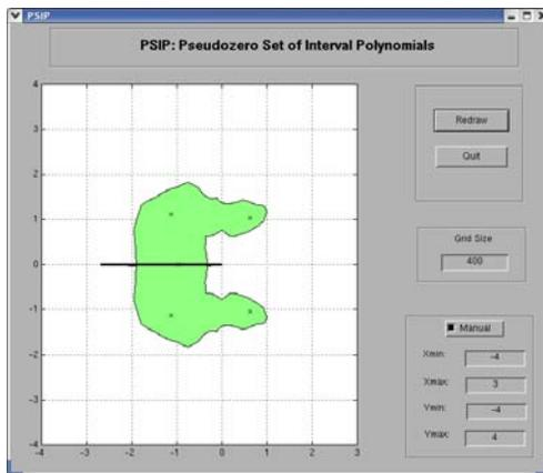
**Figure 3: Graphical User Interface of PSIP with the pseudozero set of the interval polynomial**  $p(z) = z^5 + [1.20, 2.73]z^4 + [1.14, 3.15]z^3 + [0.20, 2.35]z^2 + [1.52, 6.21]z + [0.15, 7.11]$
