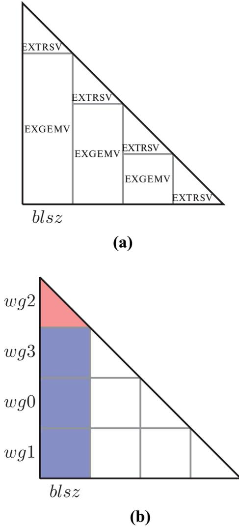
**Figure 3.** Partitioning of a lower triangular matrix  $L$ , where  $blsz$  stands for a block size and  $WGx$  is the number of a workgroup  $x$ : (a) kernel wise and (b) work group wise.
