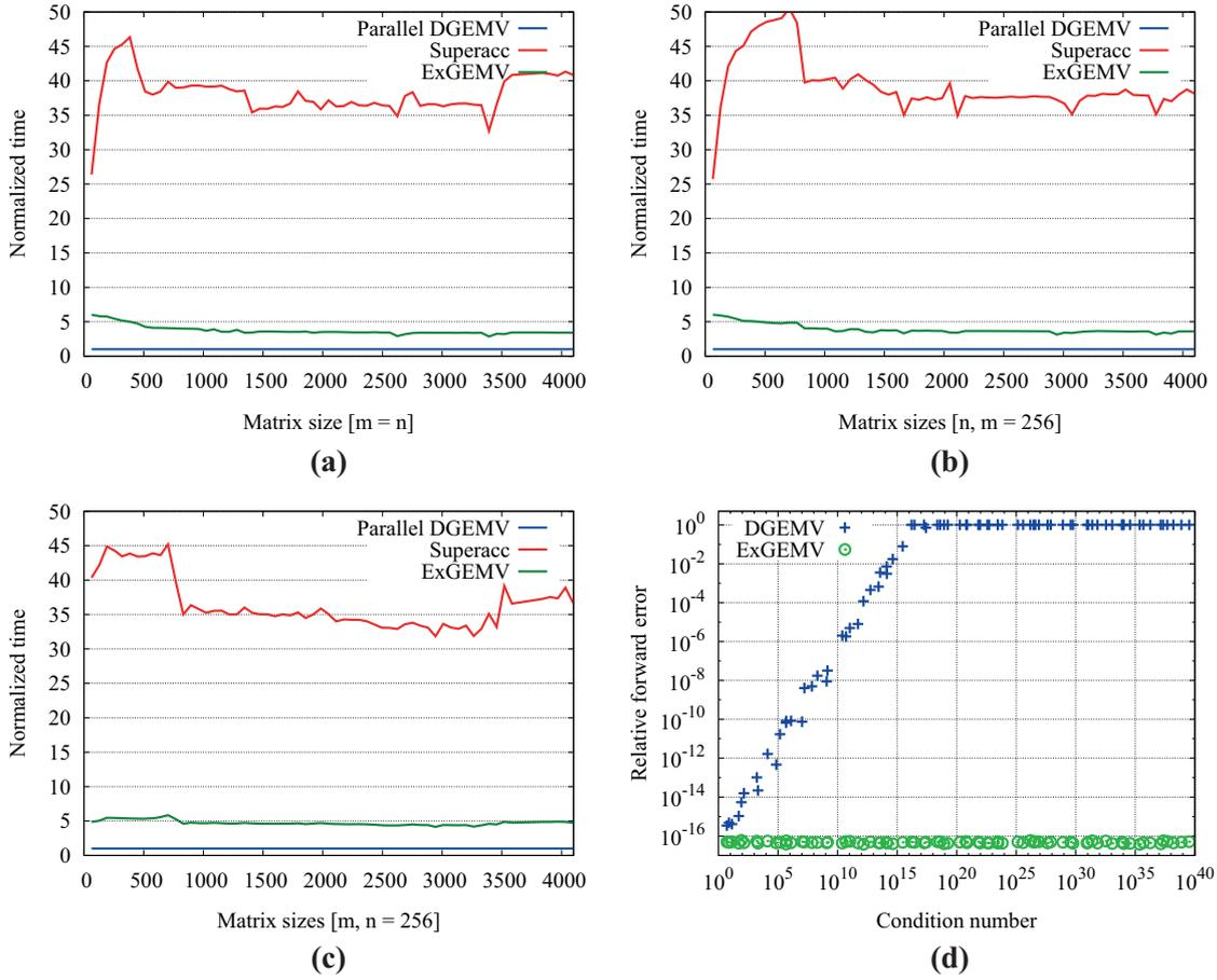
**Figure 5.** Performance and accuracy results of GEMV: (a) GEMV ( $m = n$ , step = 256) on K80, (b) GEMV ( $m = 256$ ,  $n$ ) on K80, (c) GEMV ( $m$ ,  $n = 256$ ) on K80, and (d) Accuracy of GEMV.
