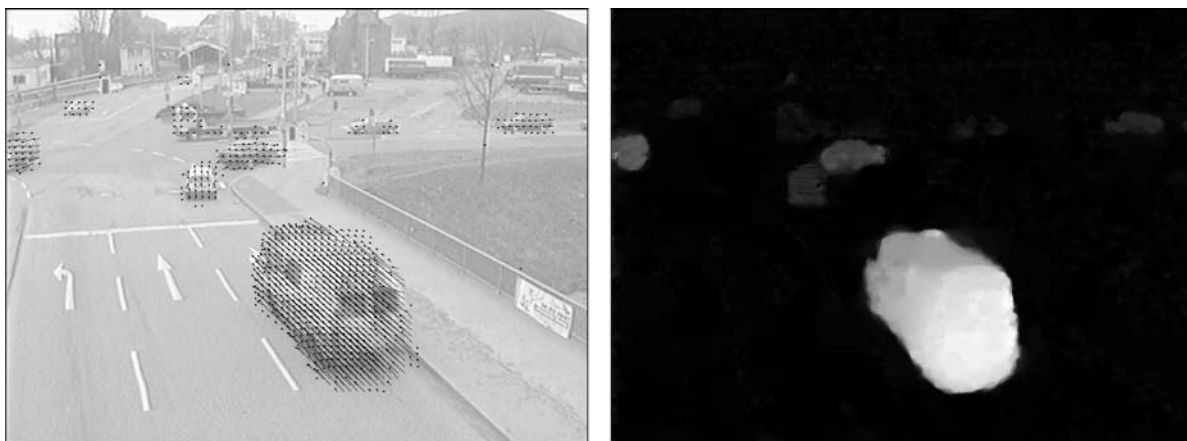
Figure 7. (a) Left: Computed flow field between frame 860 and 861 of the Karl Wilhelm Street traffic sequence. (b) Right: Computed magnitude of the optical flow field.
