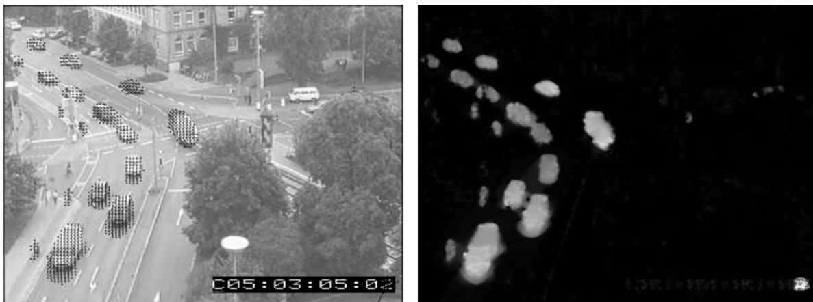
Figure 6. (a) Left: Computed flow field between frame 860 and 861 of the Karl Wilhelm Street traffic sequence. (b) Right: Computed magnitude of the optical flow field.
