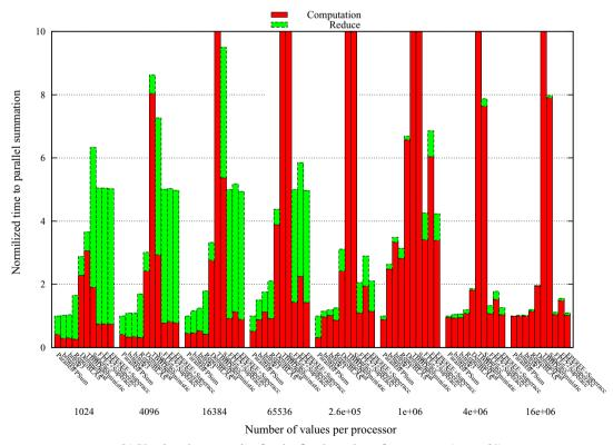
(b) Varying the array size for the fixed number of processors (np = 64).
