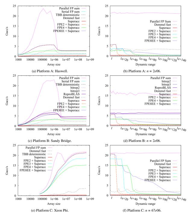
Fig. 4. The summation performance results on modern desktop and server Intel CPUs as well as the Intel Xeon Phi co-processor, see Table 2; Gacc/s stands for billions of accumulations per second.
